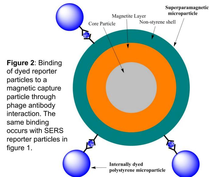
**Figure 2:** Binding of dyed reporter particles to a magnetic capture particle through phage antibody interaction. The same binding occurs with SERS reporter particles in figure 1.
