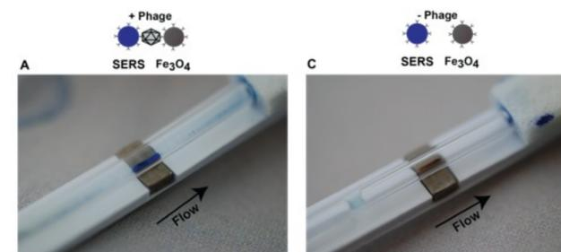
**Figure 4:** LFCC phage complex test. A: Phage positive test gives a positive, blue line over the magnet. B: Raman spectrum of SERS reporter particles. C: Phage negative test gives a negative, brown line over the magnet.
