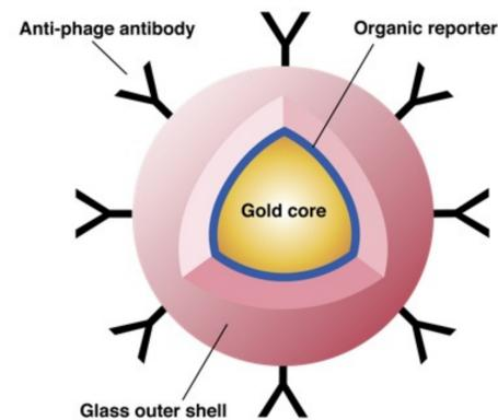
**Figure 1:** SERS Oxonica Nanoplex Biotags have a gold core surrounded by an organic reporter which has a unique Raman profile. There are a variety of reporters that give different Raman spectra. The glass outer shell is thiolated, which allows for antibody conjugation to the surface of the particle.[2]
